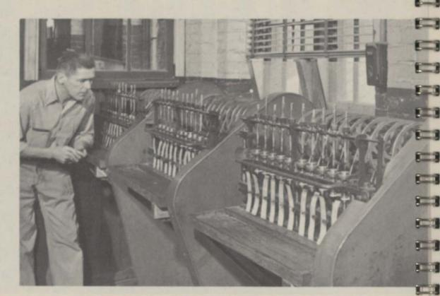
Wire drawing dies, tungsten carbide or industrial diamond, are encased in steel to withstand the great pressure of the elongation process during the wire drawing operation. Here machines recut diamond dies. The diamond die maker is checking the dies being recut to make certain each one is centered correctly for perfect roundness of hole diameter.
