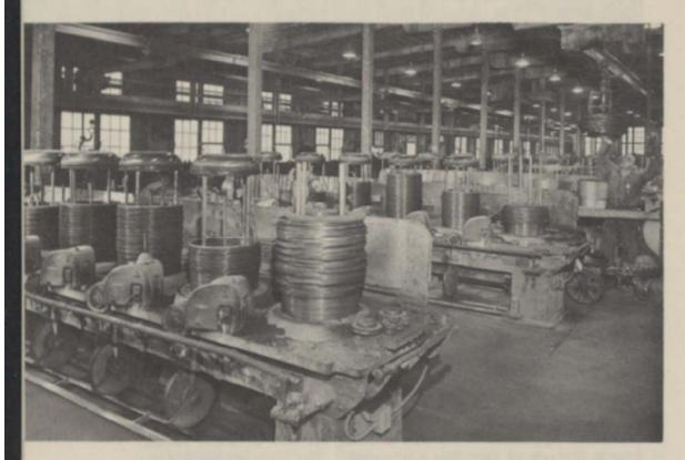
The operator is lowering a finished 200 lb. bundle to buggy for delivery to heat treating or galvanizing department for further processing.
