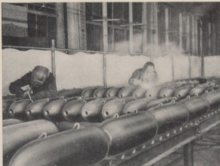
WELDING SUSPENSION LUGS ON CASINGS
