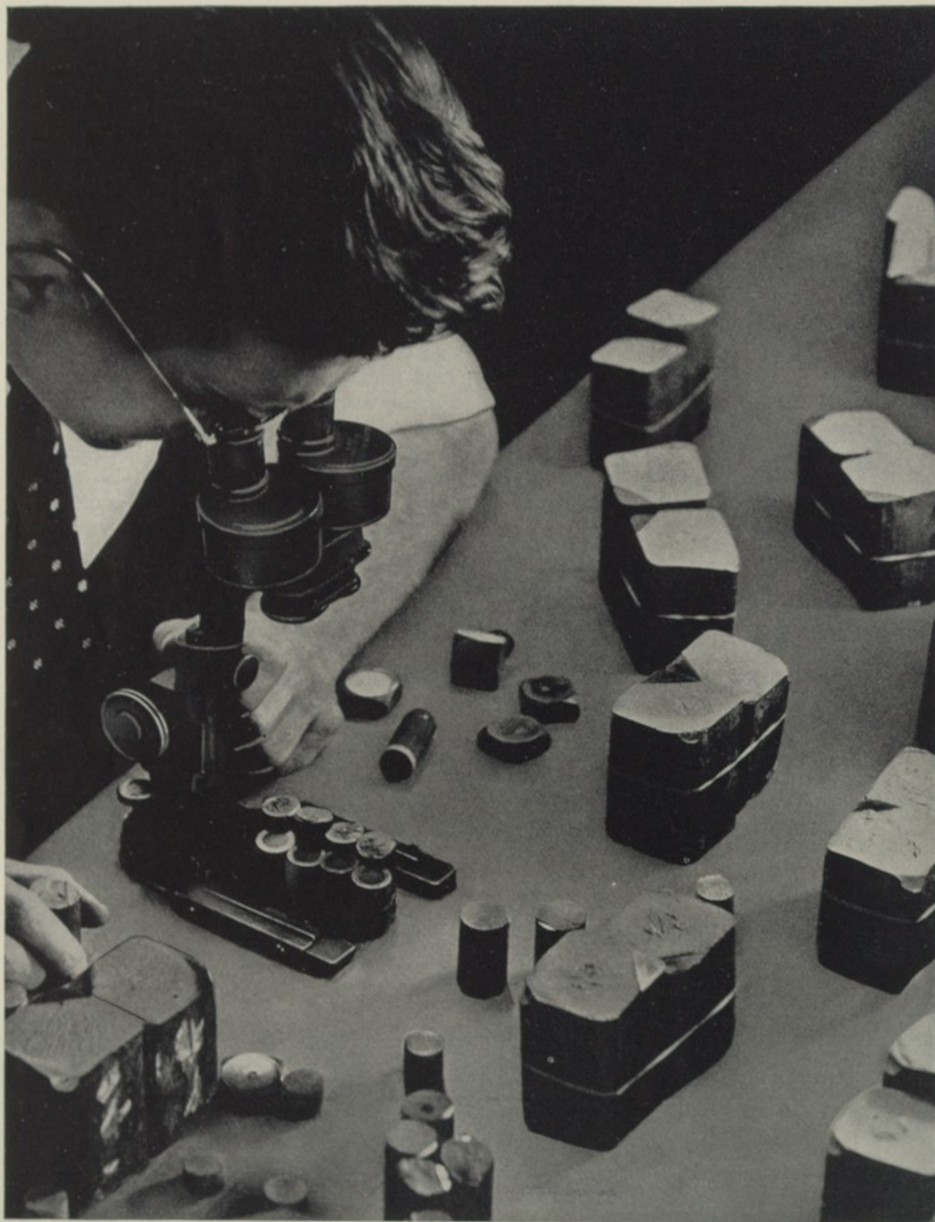
Chemical and microscopic research aid the steel industry to produce quality products. With a binocular microscope, a laboratory worker examines the grain structure of steel to determine effects of heat treatment.
