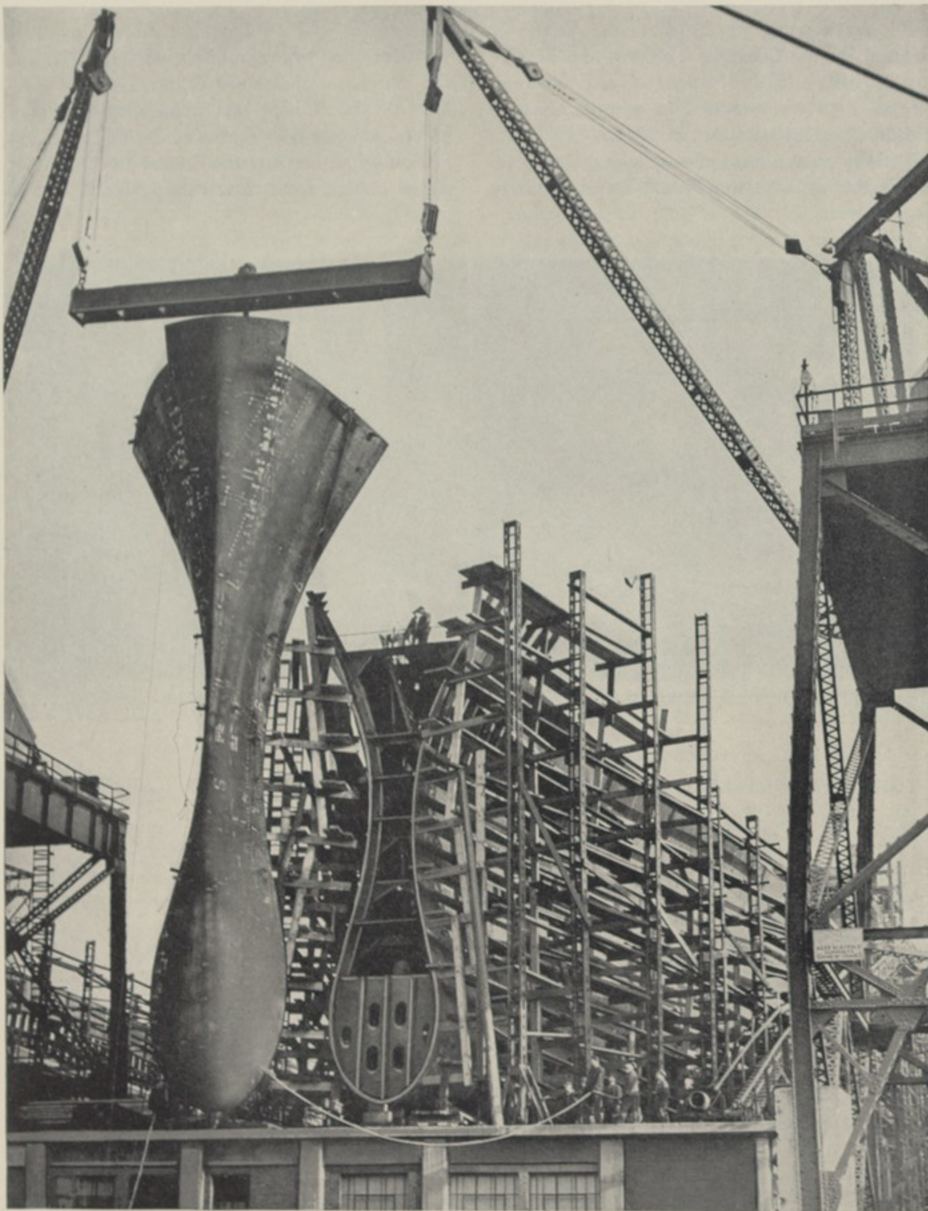
A welded bow section of a new tanker being erected on a shipway. The assembly of large hull units in the shop constitutes one of the modern methods of speeding-up the emergency shipbuilding program.
