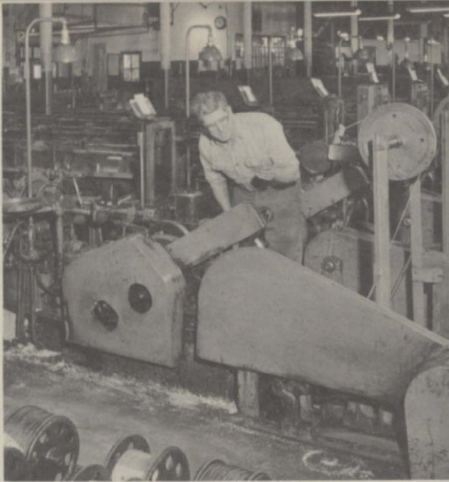
After spooling comes the stranding operation—twisting a number of wires around a center wire. Here, operator is inspecting one of the smaller stranders that revolves at very high speed. These machines produced millions of feet of aircraft control cable in World War II.
