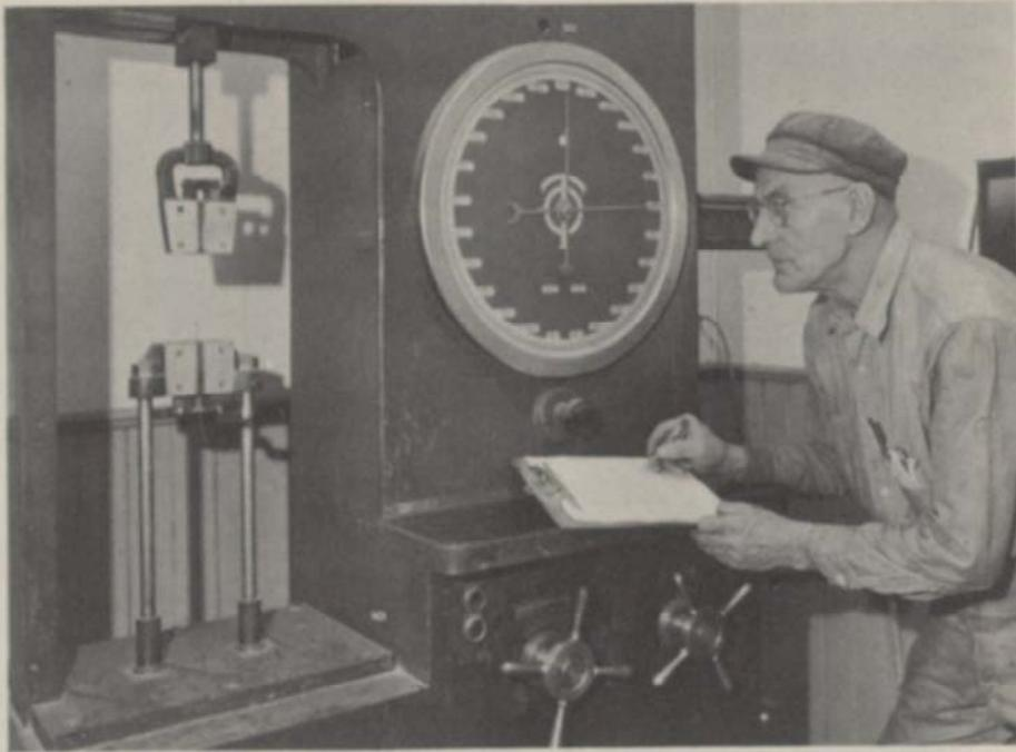
One phase of quality is control testing which determines the strength of wire. The tensile testing machine pulls a sample of wire until it breaks and the breaking strength is recorded. Metallurgical process observers, trained in the techniques of testing wire, accumulate test data to be used as a basis for the quality control.
