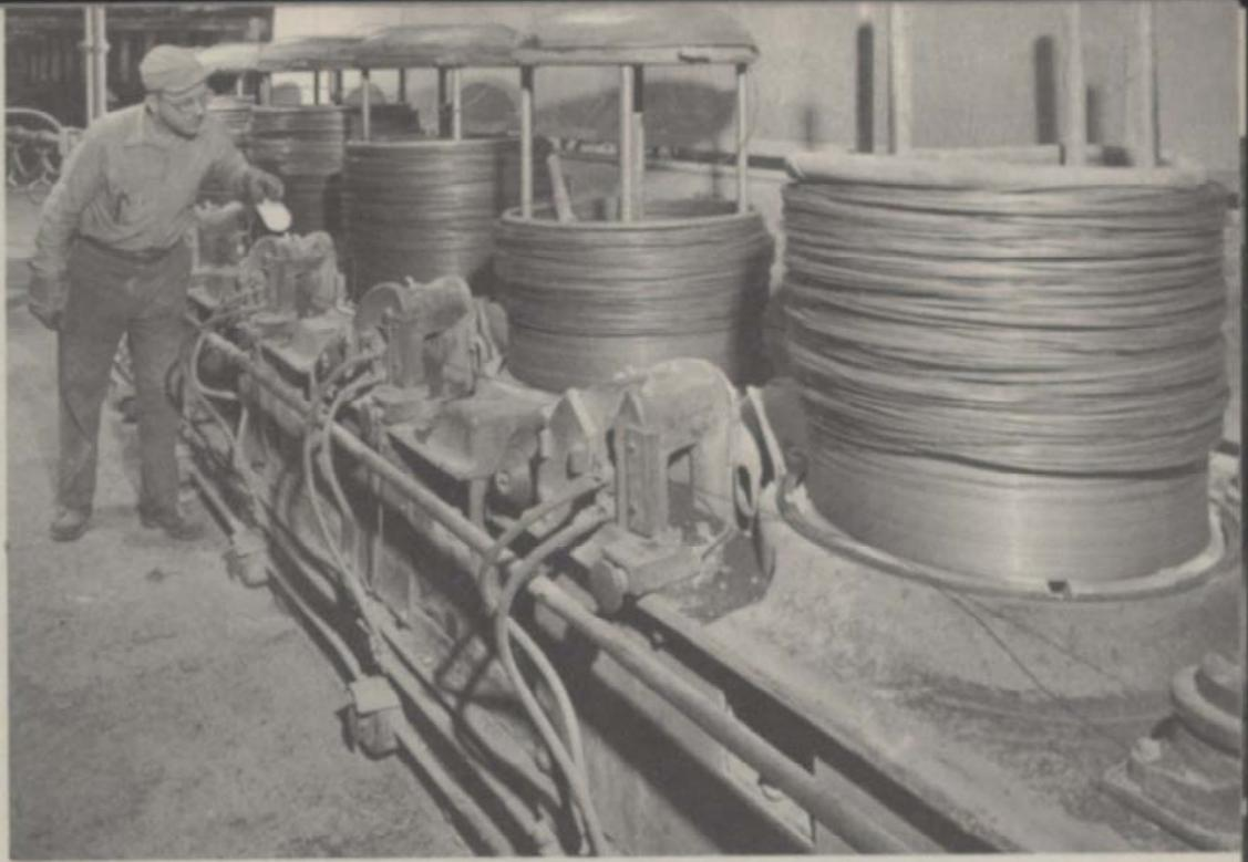
High carbon rods drawn 4, 5 or 6 reductions to finished size in one continuous operation. This wire drawing machine produces finished wire at the rate of 1500 feet per minute. The tungsten carbide dies are water cooled.
