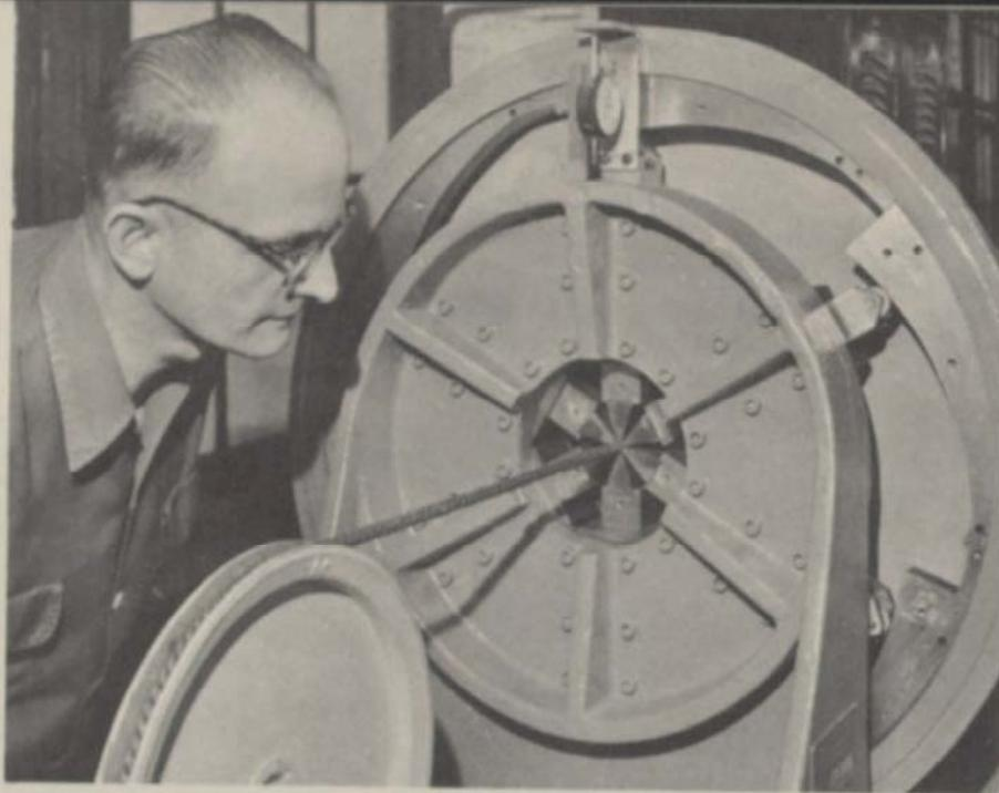
Jute, Java, Sisal, Hemp, Cotton Fibre centers undergo rigid inspection in the fibre center testing. Six jaws representing the outer steel strands of a wire rope can be interchanged for testing various sizes. This machine subjects the material to the type of treatment it will receive when it becomes the center of actual wire rope. Because the center is the heart of rope, this inspection is vital.
