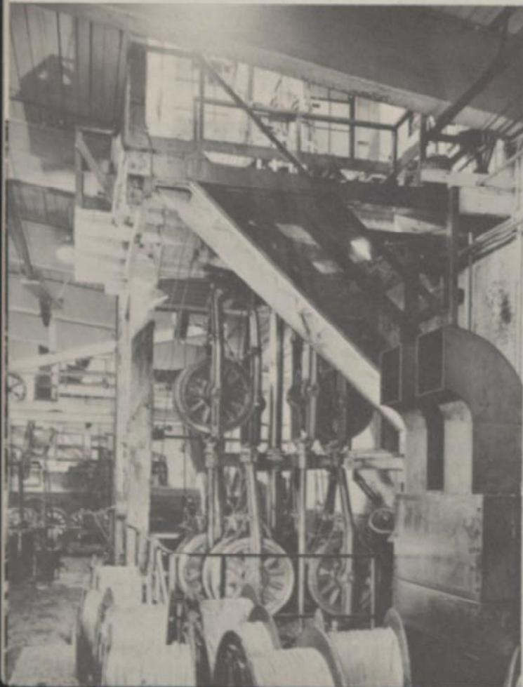
Here are two types of machines that lay the wire strands into wire rope in accordance with exacting standard practice specifications set up by rope engineers. These rigid standards assure quality that must pass tests for breaking strength, bending fatigue, resistance to wear, twisting characteristics. In the *foreground*, vertical layer; *background*, horizontal type.
